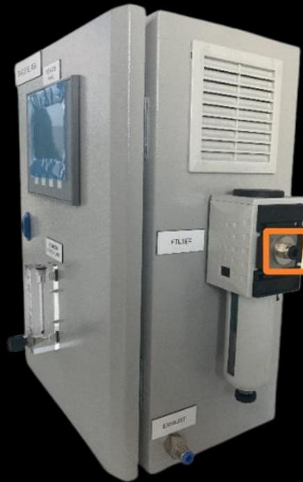
The filter has a manual unloading system. You must follow as periodically. Suggested, depending on processes once a week. The input pneumatic hose is 6mm in diameter.
