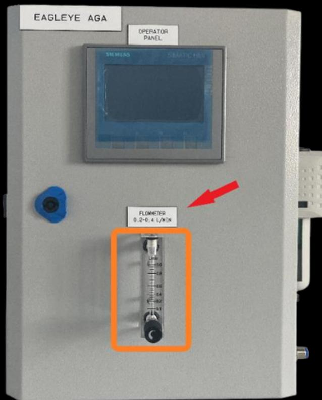
The flow must be within 0,2-0,8 lit/min. When the analyzer works, the calibration tubes, or sample line must be this flow range. The flow range is marked with a red arrow on the panel.
